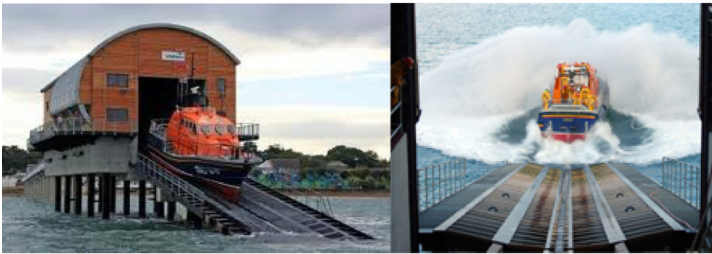
Fig. 6. The launch process of RNLI lifeboat from a slipway station.
