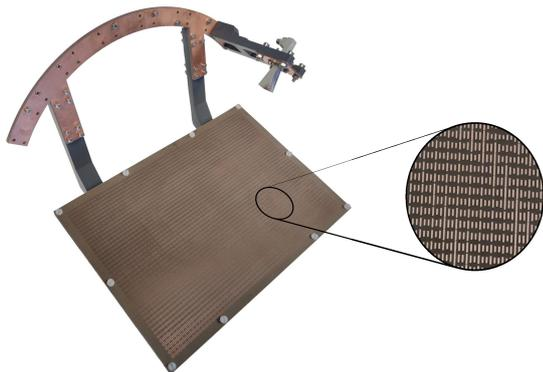
Fig. 4. Reflectarray antenna demonstrator with beam steering using a tilted focal arc.
