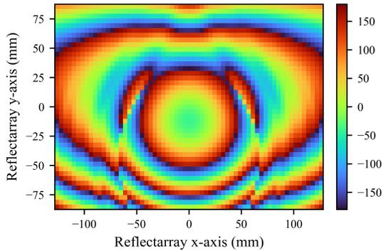
Fig. 3. Selected phase shift distribution for the manufactured antenna prototype.
