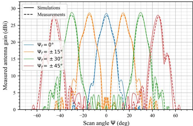
Fig. 5. Measured antenna gain within the scanned plane for multiple feed positions.
