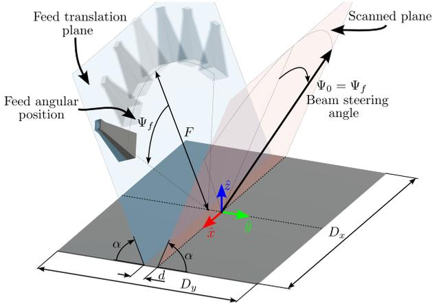
Fig. 1. Mechanically steering RA antenna optics based on a tilted focal arc. The feeding horn models are merely illustrative.
