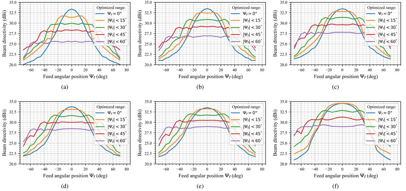
Fig. 2. Estimated steered beam directivity for multiple compactness levels and steering ranges. (a) through (e) represent the beam steering performance for tilted focal arcs of radi  $F = \{0.55, 0.7, 0.85, 1, 1.15\}D_y$ , respectively. (f) presents the same results for a centered arc configuration (i.e.,  $\alpha = 0^\circ$  and  $d = 0$  mm) with  $F = D_y$ .
