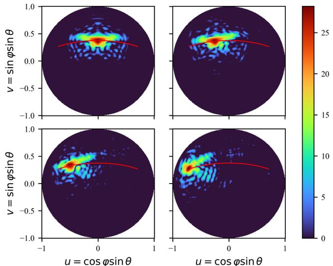
Fig. 6. 3D measured gain patterns for beam positions  $\Psi_0 = 0^\circ$  (top left),  $\Psi_0 = 15^\circ$  (top right),  $\Psi_0 = 30^\circ$  (bottom left) and  $\Psi_0 = 45^\circ$  (bottom right). The red line represents the projection of the scanned plane.
