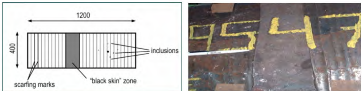
Fig. A3.14: Dimensions and photograph of the slab sample used to test different inspection devices
