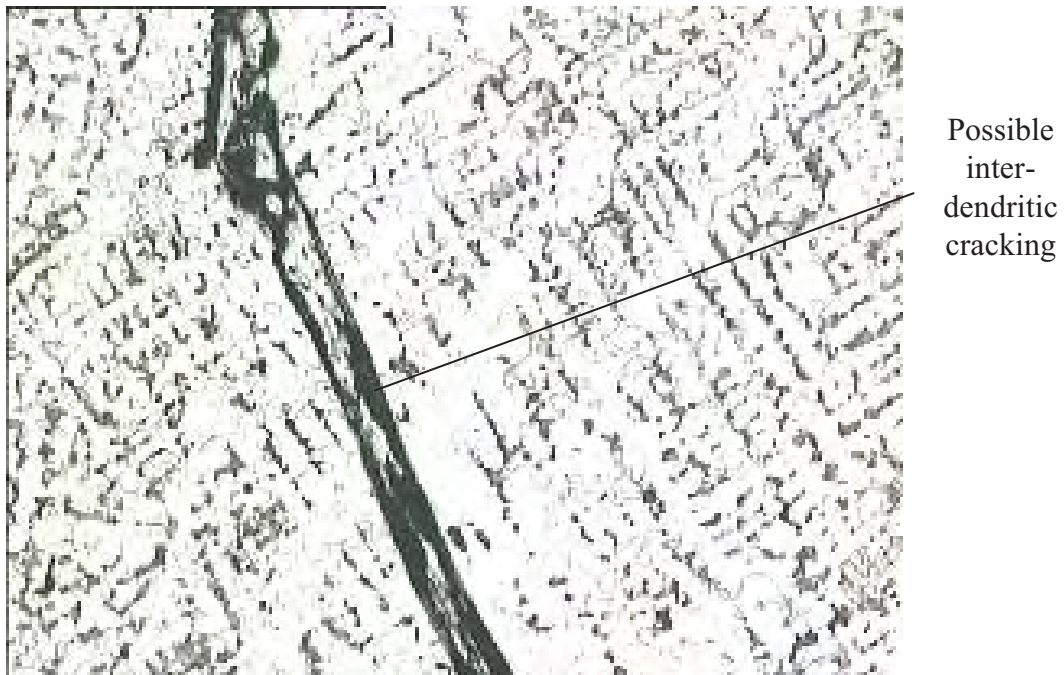
Fig. A4.22: Cross-section and microstructure of crack, cast 60942, slab 5B, sample 5, after etching, x100
