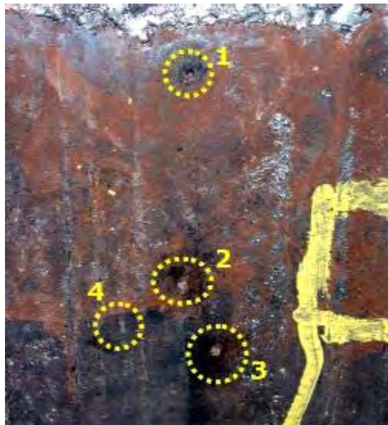
Fig. A3.15: Part of the slab sample used to test different devices for inclusion detection. Pore 1 had a diameter and a depth of 3 mm*0.7 mm. Pore 2 measured 5 mm*2.3 mm, Pore 3 measured 4 mm*0.7 mm and Pore 4 measured 1.5 mm*0.4 mm.
