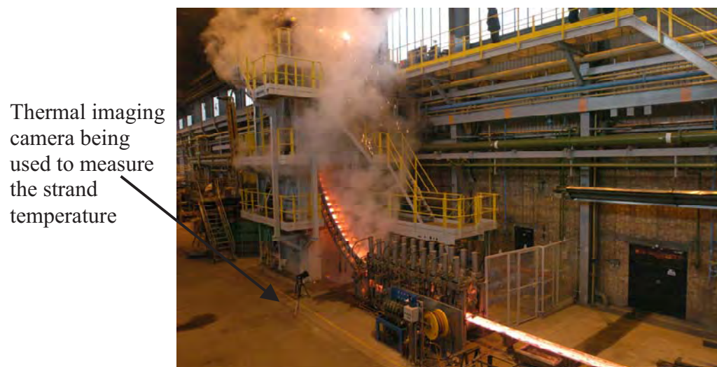
Fig. A1.78b: Side view of the continuous caster at Teesside Technology Centre
