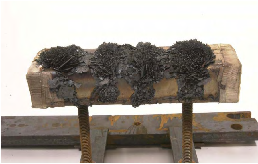
Fig. A1.24: Photograph of the scale collector, with scale piles on top of each of the four magnets housed inside the box
