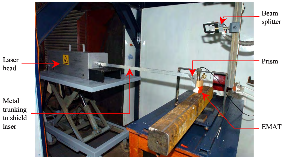
Fig. A1.29: The portable laser system, positioned above the billet being tested at Corus Teesside Technology Centre
