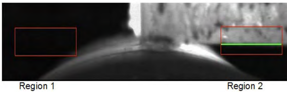
Fig. A3.2: The image of the roll area selected by the CMOS camera. The rectangle areas represent the two parts the camera examines and compares
