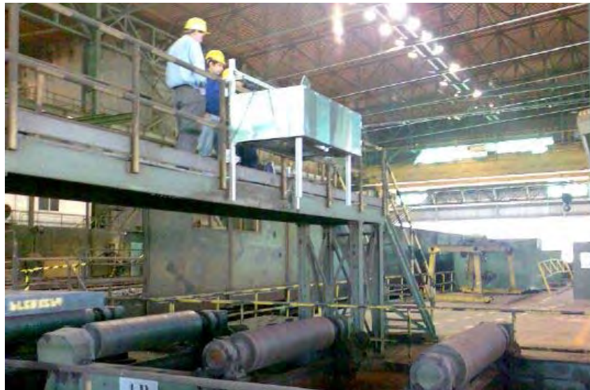
Fig. A3.10: The new line scan optical system inspecting scarfed slabs in the Arcelor plant
