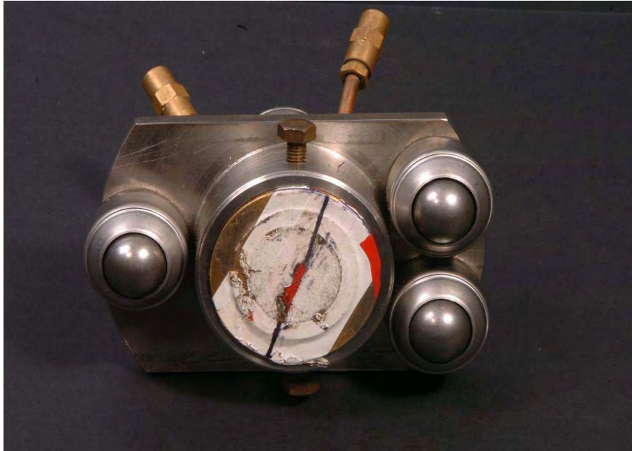
Fig. A1.28: The water-cooled EMAT mounted in a tripod
