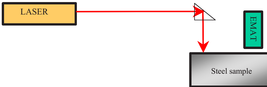
Fig. A1.30a: Apparatus arrangement with no prism present
