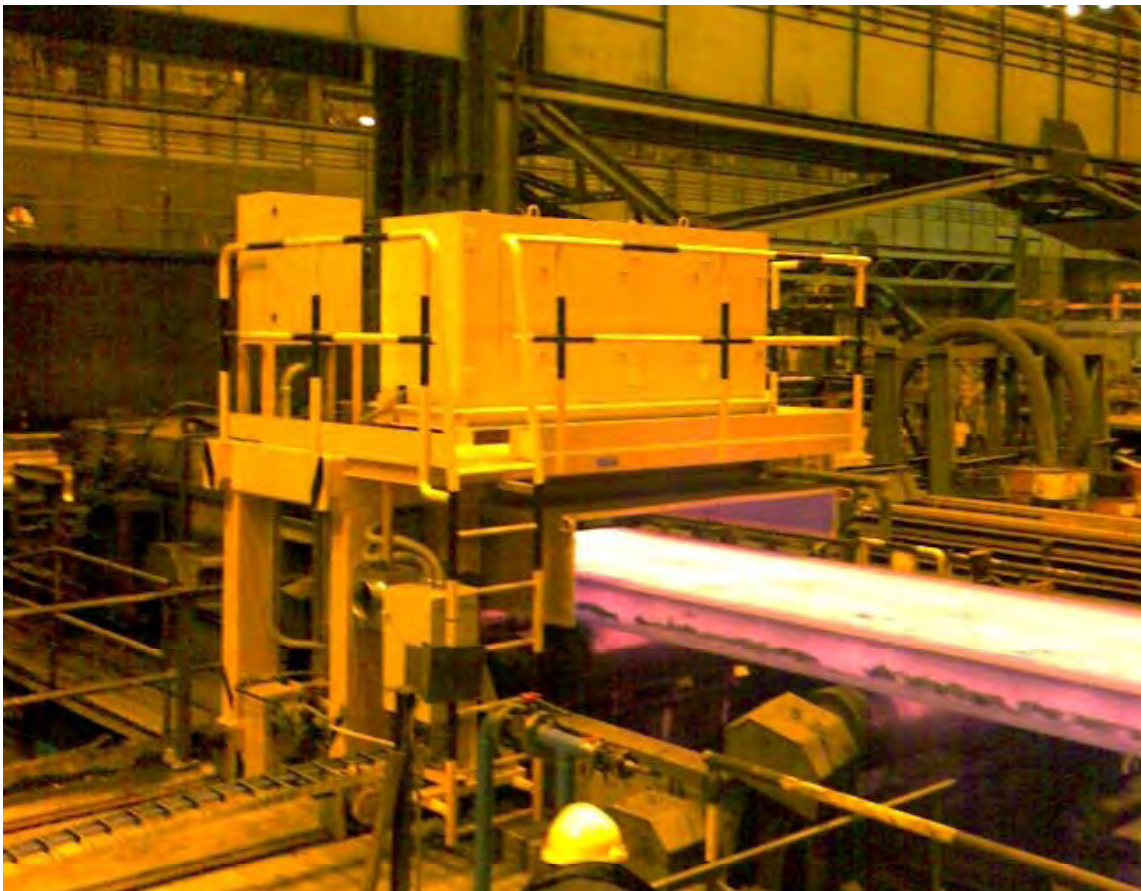
Fig. A2.12: External view of the final surface inspection system in operation on the steel plant
