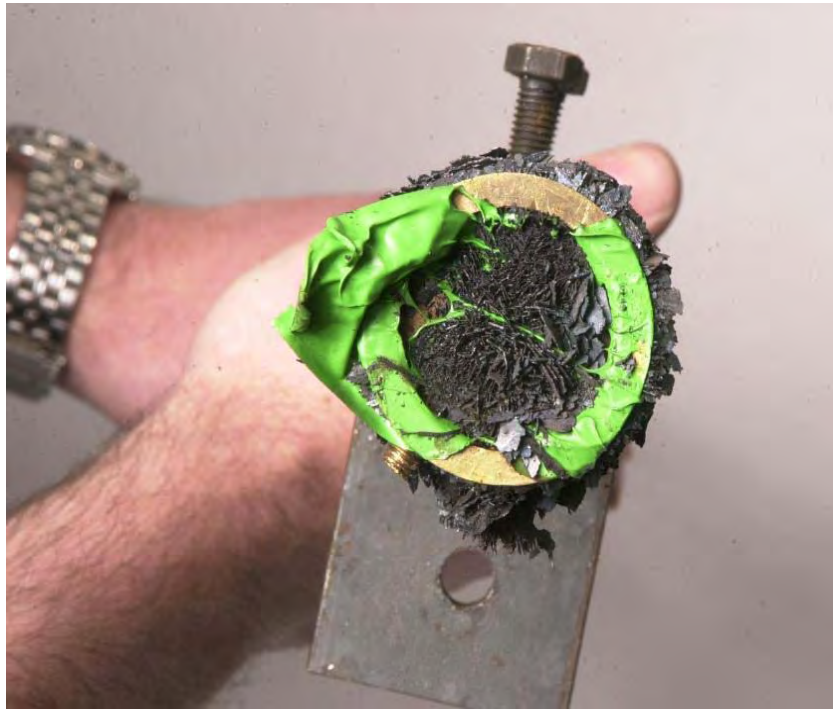
Fig. A1.22: The build up of scale on the EMAT face
