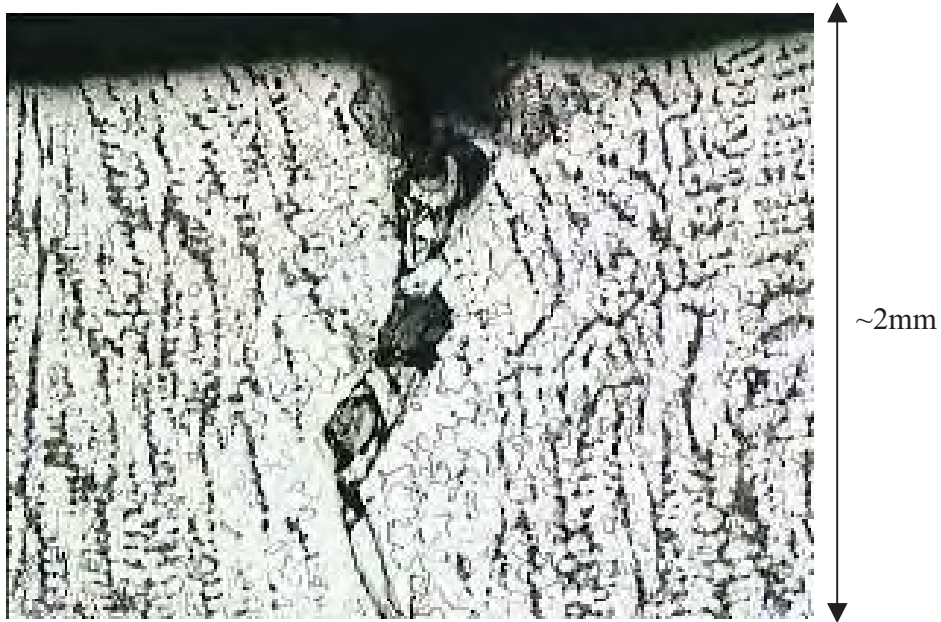
Fig. A4.16: Cross-section and microstructure of crack networks, cast 60933, slab 5B, sample 1, after etching, x50
