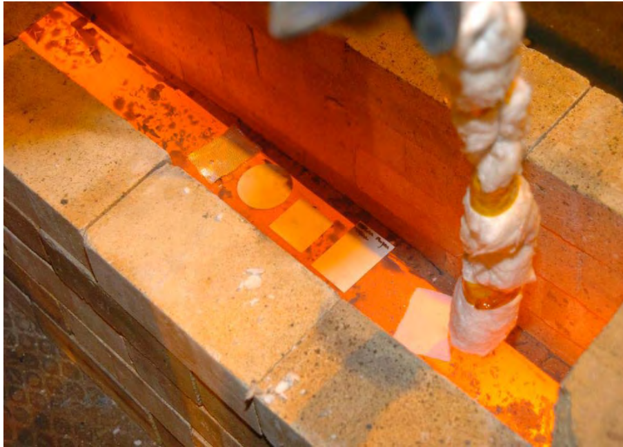
Fig. A1.69: A longer billet sample being used to test different ceramic tiles
