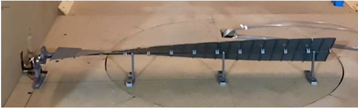
Fig. 18. Twisting of the Benchmark model in developed torsional instability.
