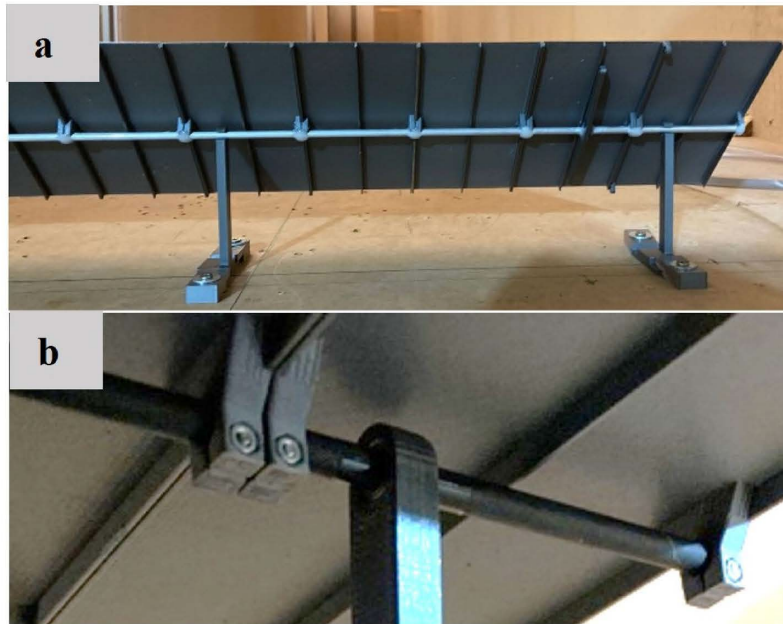
Fig. 4. Assembly of the panels, torque tube and pillars: a) general view; b) detail of the version with bearings and screw clamping.
