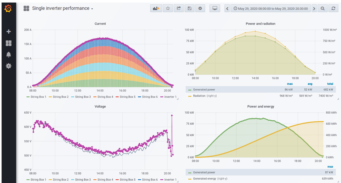
Fig. 9. Monitoring dashboard of an inverter on Grafana. Data is extracted from Kapua database to Grafana graphics to improve the quality of the monitoring.
