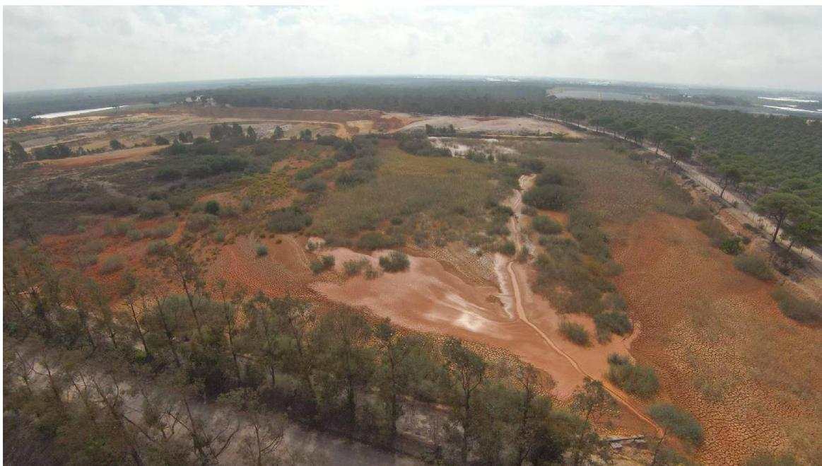
**Figure 1.** Image of the ponds in which sludge from aggregate washing is deposited.
