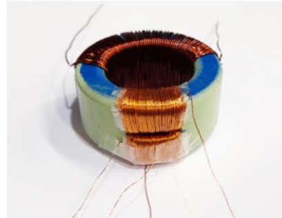
Fig. 9. The constructed variable inductor based on the toroidal-cut magnetic core.
