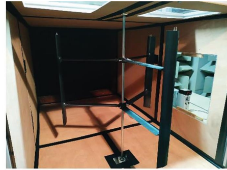
FIGURE 1: Aerodynamic enclosure with the turbine in the wind tunnel.
