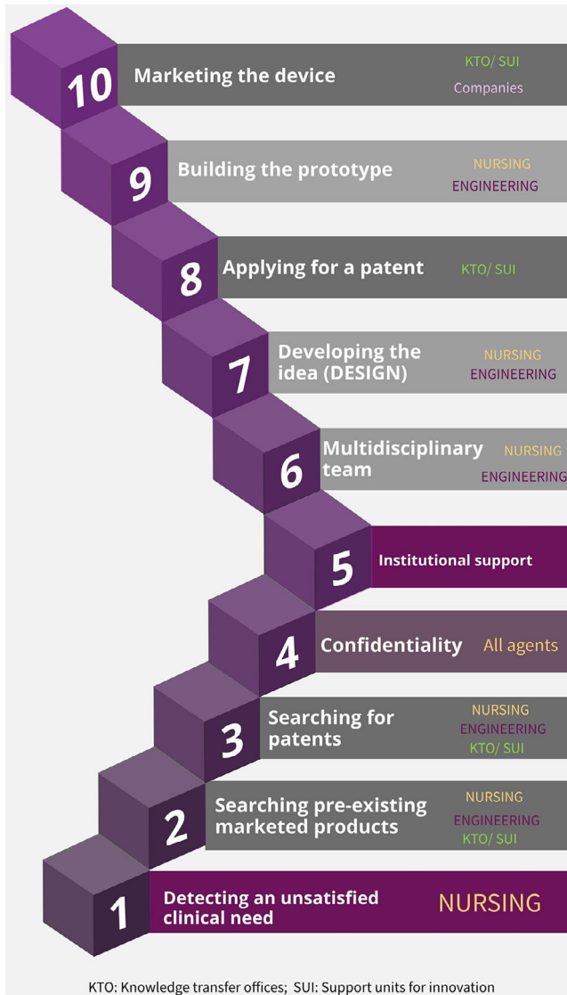
FIGURE 2 Ten-step process for design of a device and protection of the invention.
