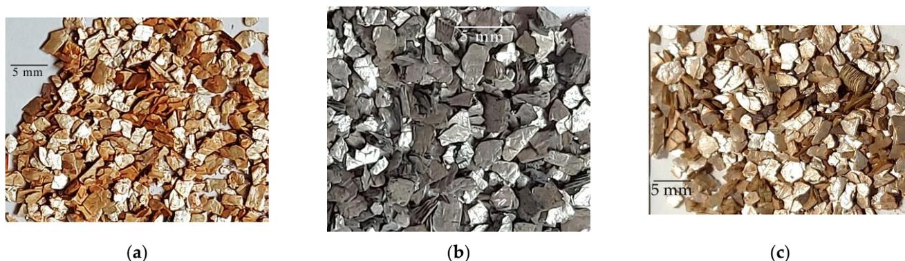
**Figure 2.** Appearance in hand sample of the vermiculites U treated in situ at 1000 °C and (a) in ambient atmosphere, (b) in reduced atmosphere of 5%H<sub>2</sub> and 95%Ar, and (c) in reduced atmosphere of 100% H<sub>2</sub>.
