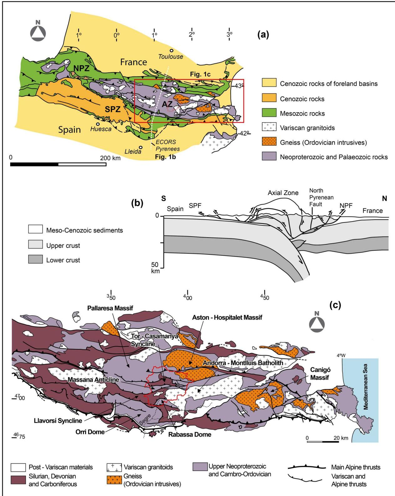
**Figure 1.** (a) Geological sketch of the Pyrenees with the location of the ECORS – Pyrenees profile (Figure 1b) (b) Geological interpretation of the ECORS Pyrenees seismic profile, from Muñoz (1992); AZ, Axial Zone; SPF, South Pyrenean front; NPF, North Pyrenean front. (c) Geological sketch of the Eastern Axial Pyrenees with indication of the main structures and the Andorra border in red, modified from Casas & Fernández, 2007.
