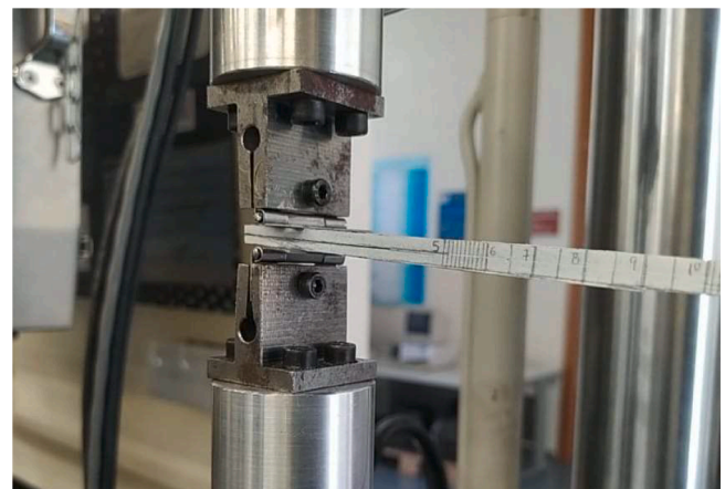
Fig. 2. Specimen arrangement on the testing machine for mode I tests.
