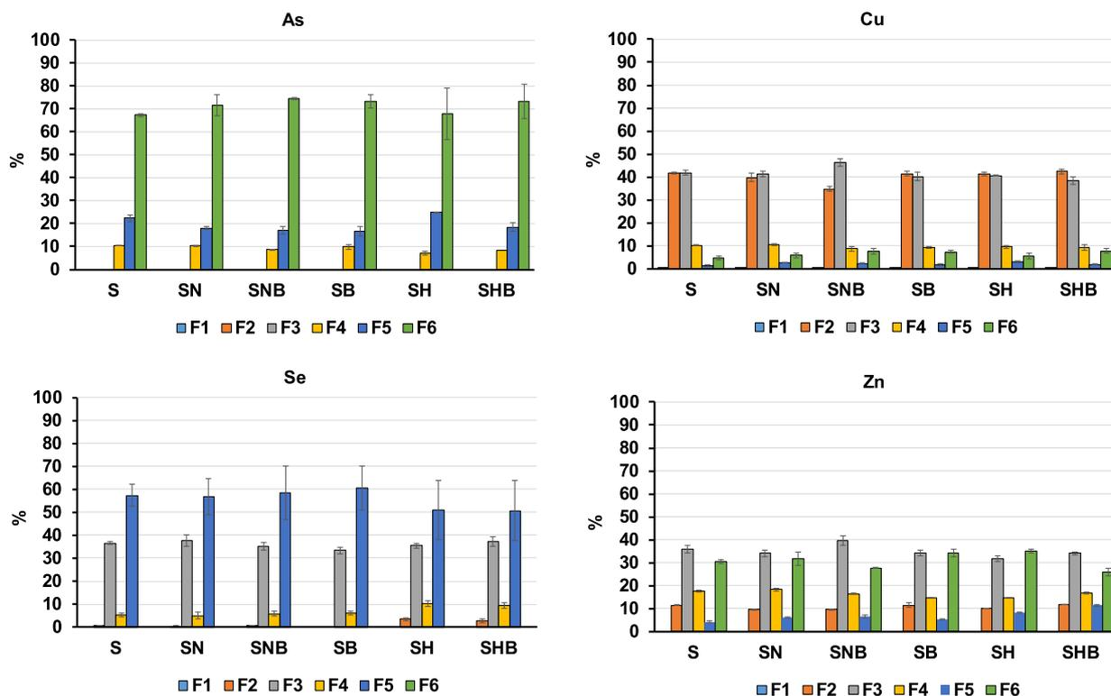
Fig. 3. Percentage of As, Cu, Se, and Zn in each fraction in the untreated mine soil and the soil with the different treatments applied. Values calculated from the data are shown in Table S1 – Supplementary material. (S: Soil. SN: Soil + nZVI. SNB: Soil + nZVI + biochar. SB: Soil + biochar. SH: Soil + nH. SHB: Soil + nH + biochar).
