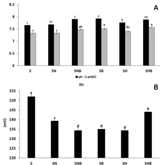
**Fig. 1.** (A) pH and pH<sub>(KCl)</sub> and (B) redox potential (Eh) in the control soil (S) and the soil treated with NPs and/or biochar. (S: Soil. SN: Soil + nZVI. SNB: Soil + nZVI + biochar. SB: Soil + biochar. SH: Soil + nH. SHB: Soil + nH + biochar). Different letters mean significant differences ( $n = 3$ , ANOVA;  $p < 0.05$ ). Data correspond to mean and error bars represent the standard deviation.
