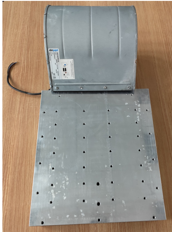
Figure 5-8: Active heat sink
