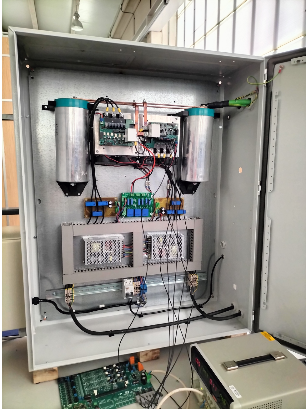
Figure 4-26: Developed back-to-back converter during preliminary tests
