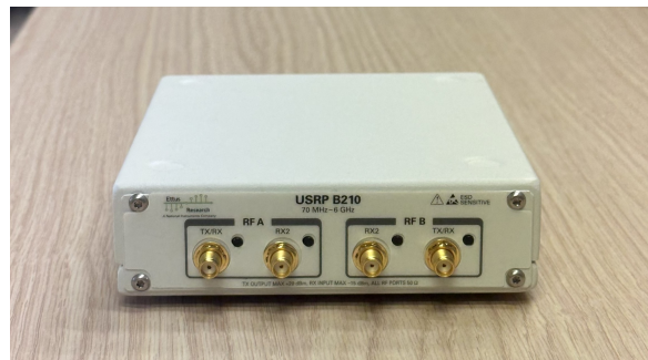
Figura 2.2: USRP B210. Fuente: https://www.ettus.com/all-products/usrp-b200-enclosure/
