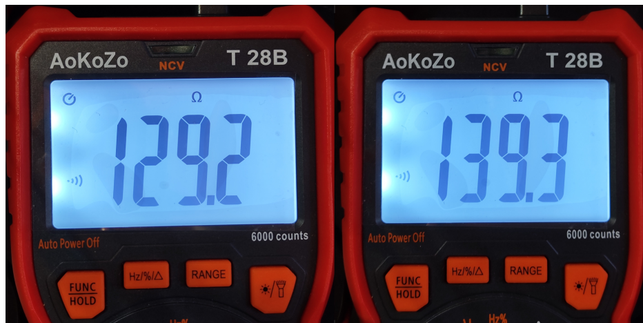
Figure 4.4: Left is band electrode to band socket, right is band electrode to 3.5 jack connector.
