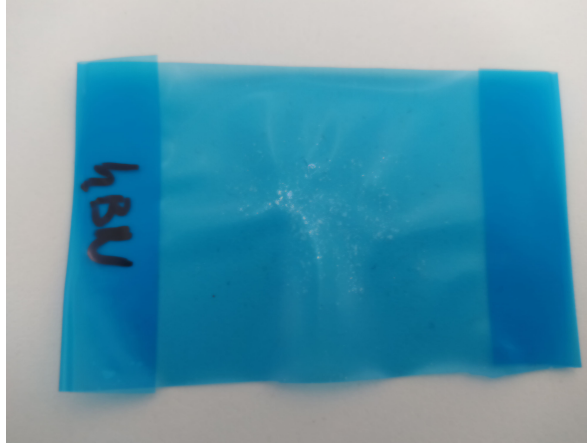
Figure 23: Blue Nitto Tape with 2D hBN crystals exfoliated on top.
