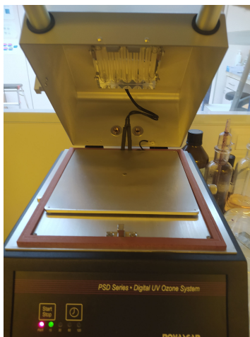
Figure 24: Ozone generating system using UV lamp
