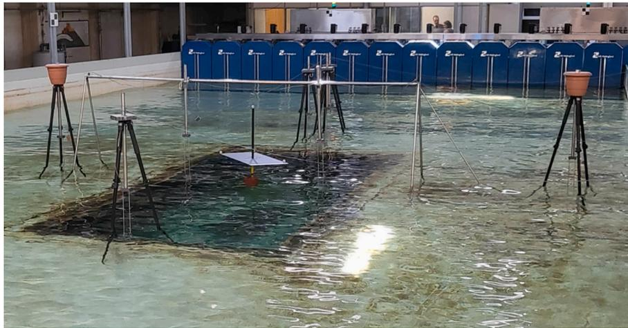
Fig. 6. Wave probes and device in the wave basin.
