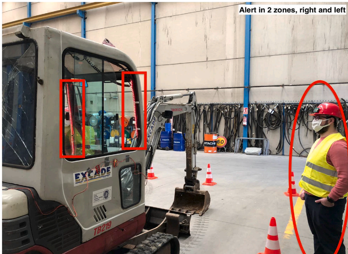
Fig. 14. Alert sign with red LED and haptic feedback.
