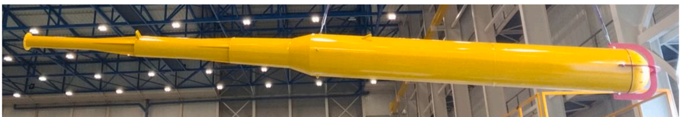
Fig. 4. WindCrete manufactured prototype hung by lugs at the FIHAC facility.
