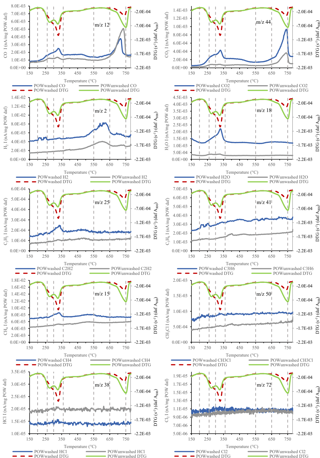
Fig. 4. Intensities (I) of carbon monoxide (CO), carbon dioxide (CO 2 ), hydrogen (H 2 ), water (H 2 O), acetylene (C 2 H 2 ), propene (C 3 H 6 ), methane (CH 4 ), chloro-methane (CH 3 Cl), hydrogen chloride (HCl) and chlorine (Cl 2 ) during POW washed and POW unwashed pyrolysis.
