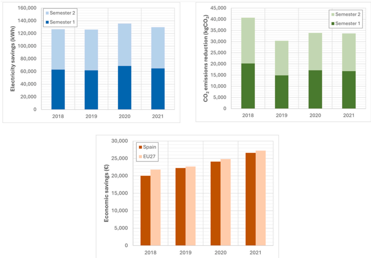
Fig. 4. Savings achieved through the reform of the lighting installation.
