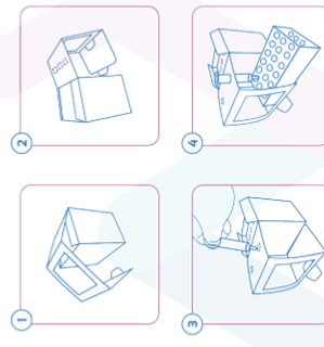
Figure 1. Graphic instructions to use column box as well as rack, avoiding to get a specific column rack in the laboratory and facilitating the protocol.
