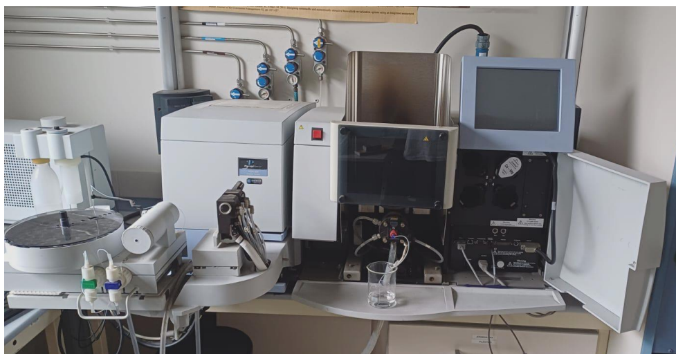
Figure 5: Perkin Elmer AA200 Spectrometer and Perkin Elmer HGA900 graphite furnace
