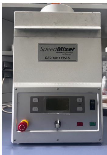
Figura 3.4.- SpeedMixer (German Engineering by Hauschild, type DAC 150.1 FVZ-K)
