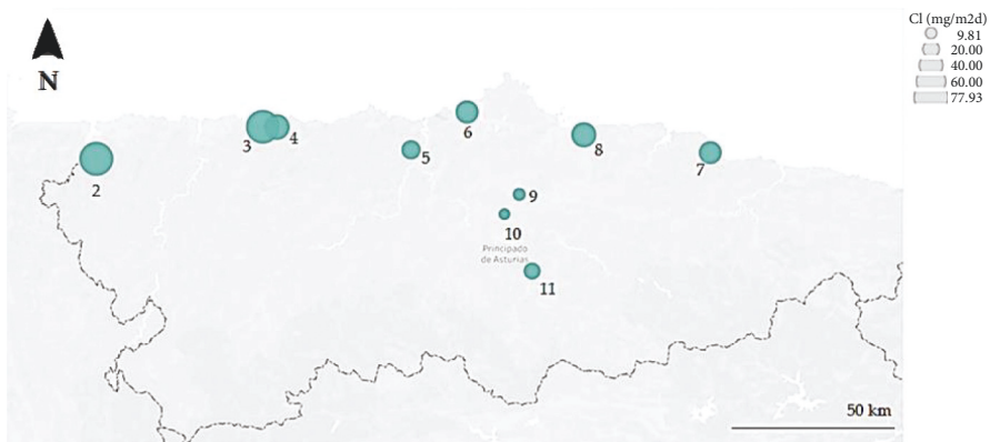
FIGURE 8: Results of test II, representation of deposition at each study location.
