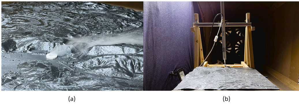
Fig. 16. (a) Detail of the particles leaving the emitting source over the orography. (b) Front view of the model with the particle emitter on with north wind.
