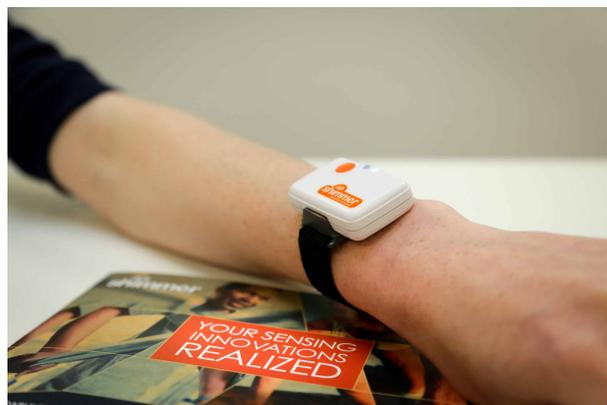
**Figura 1.2:** Sensor inercial Shimmer3. [15].
