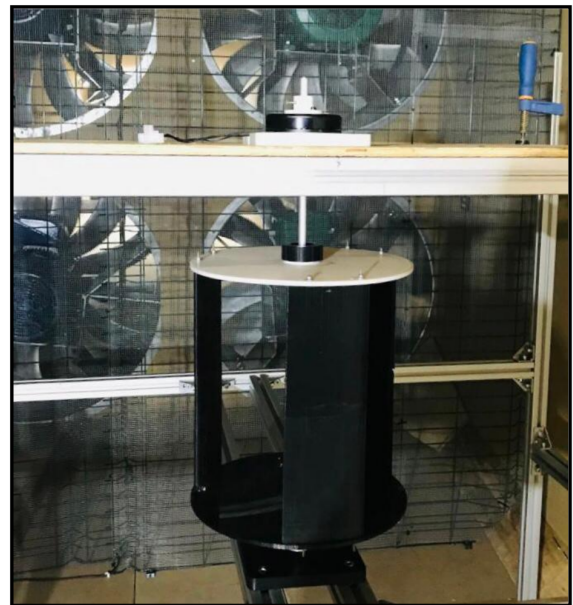
FIGURE 3: The turbine model inside the tunnel.
