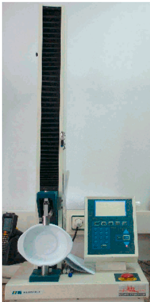
Fig. 3. Hounsfield equipment for compression and stiffness tests on trays.
