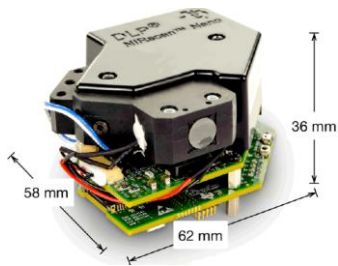
Fig. 2. Texas Instruments DLP NIRscan Nano dimensions.
