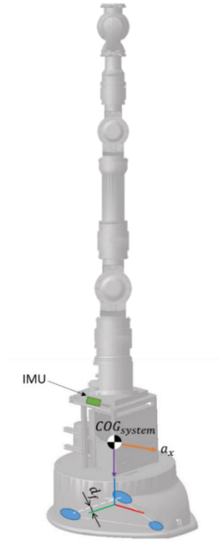
Figure 107 Robot manipulator position for the estimation of the effects of linear accelerations.
