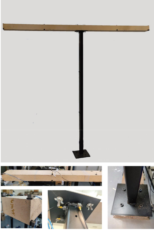
FIGURE 5: The T steel-wood structure used in the experiments.
