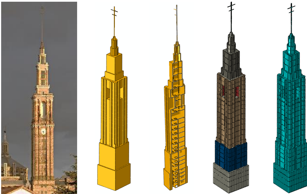
Figure 5. Details of the FEM of the Laboral city of Culture Tower.
