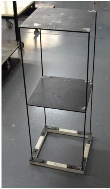
Figure 5. Two-floor steel frame structure.
