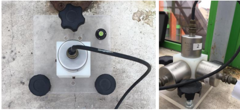
Figure 4. PCB 393B31 accelerometers
