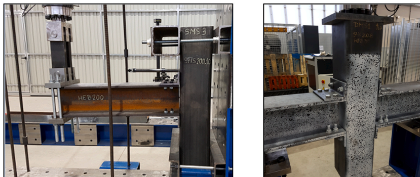
Fig. 1. Type of beam-column joint tested. (a) Beam connection to one side of the column (SMS); (b) Connection with beam on both sides of the column (DMS).
