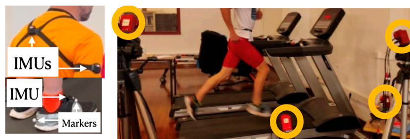
Figure 4. (Left): positioning of the IMUs, and the reflective markers for the optical MOCAP system, over the body of the athlete. (Right): Optitrack camera disposition.
