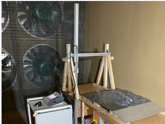
Figure 8. View of the physical model tested in the wind tunnel.
