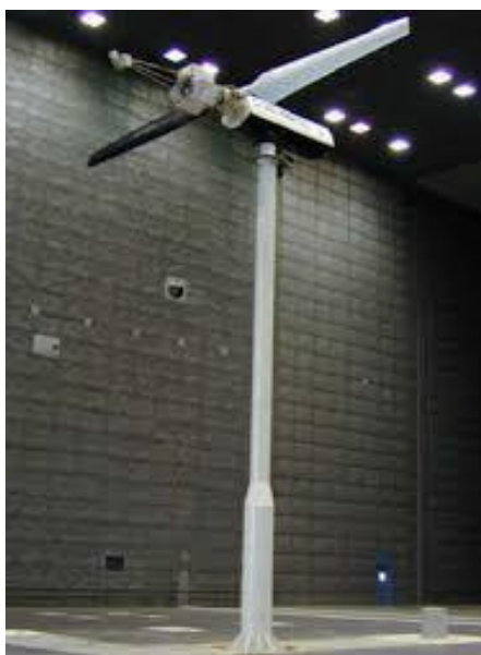
Figure 2. NREL Phase VI turbine (left), turbine blade (upper right) and S809 profile that forms the blade (lower right) [6].
