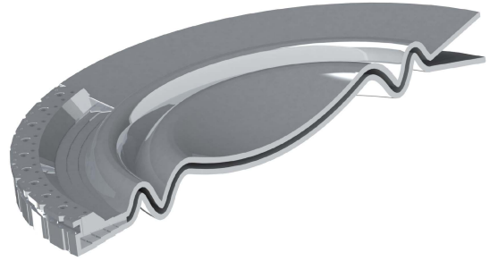
Fig. 5. Cross-section view of the AM compact and lightweight design (symmetry ground plane removed to show the inner cavity).
