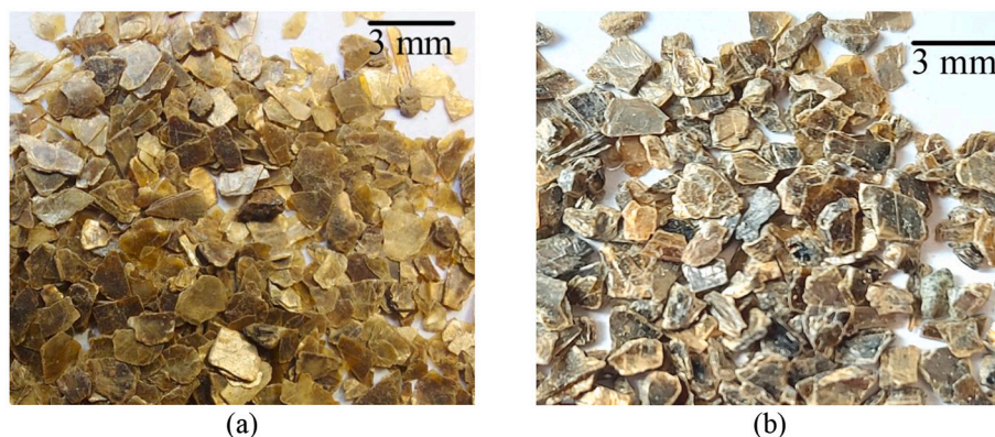
Fig. 1. Appearance of the raw vermiculites: (a) Ugandan vermiculite, (b) Chinese vermiculite.
