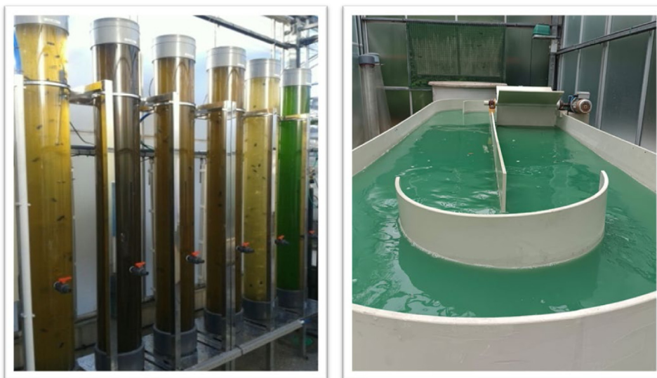
Fig. 1. Culture systems used for large volumes (left: PBRs, right: raceways).
