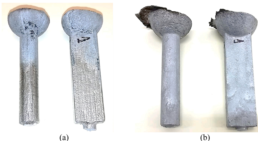
Fig. 9. Molded parts using different molds: (a) as-built mold, (b) treated mold.
