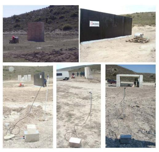
Figure 2. Charge locations in front of the different structures.
