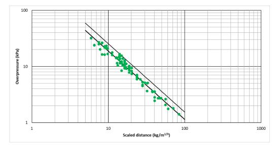
**Figure 4.** Air overpressure measured as a function of scaled distance with Riodin charges (dots are actual values while lower and upper lines correspond to Equation (3) and Equation (5) respectively).
