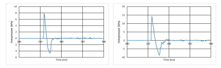
Figure 3. Air overpressure measured in tests no. 17 (left) and no. 37 (right).
