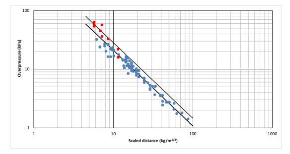
**Figure 8.** Overpressure measured as a function of scaled distance for the detonation of pure TNT and equivalent TNT (dots are actual values while lower and upper lines correspond to Equation (8) and Equation (9) respectively).
