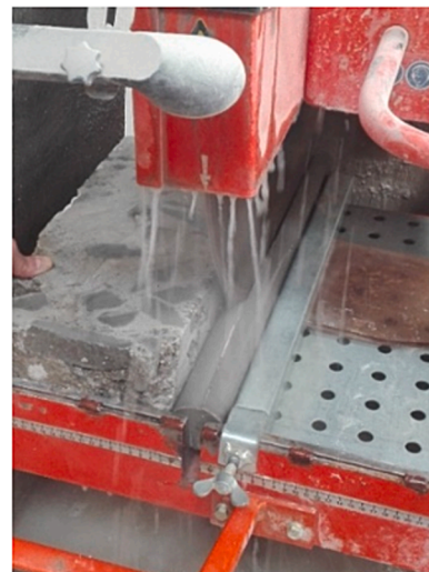
Fig. 7. a) Filling the split PVC pipe. b) Test tube cutting.
