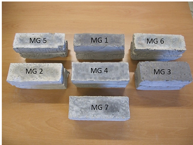
Fig. 2. Geothermal grout candidates.
