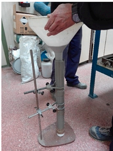
Fig. 7. a) Filling the split PVC pipe. b) Test tube cutting.
