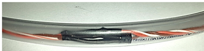
Figure 12. DS18B20 sensor on the 1-wire bus inside the protection hose.
