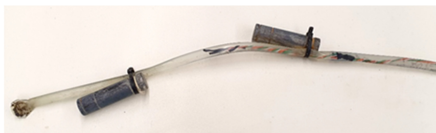
Figure 14. The 1-wire cable protected with an outer tubing and filled with oil Q-Thermie-uniovi-2.
