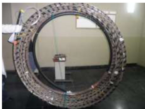
Figure 13. External geothermal pipe with temperature sensors used in Q-Thermie-Uniovi-1 borehole.
