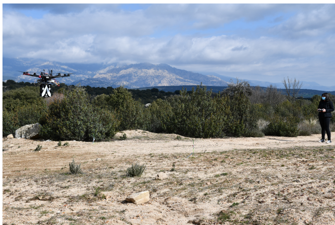
Fig. 14. UAV-based GPR prototype [58] conducting a validation test for IED detection in an scenario consisting of a dirt road.
