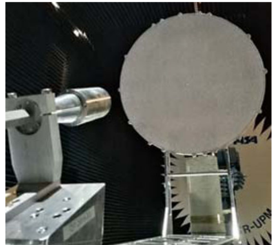
Fig. 16. Manufactured parabolic reflectarray scaled in a factor of 0.5.
